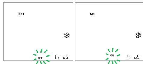
Press the UP and DOWN buttons to set the frost protection temperature. Allowable temperatures range from 5 to 15 °C (41 to 59 °F) with a default of 5 °C (41°F). Press the MODE button to confirm and continue to the next menu item.
